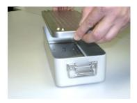
Use a small object (e.g. a screwdriver) to remove the seal from the lid groove and slide out the seal.
