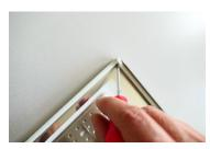
Check the old seal after removal as to whether the seal face of the lid is damaged or soiled. If necessary, clean the lid before inserting the new seal.
